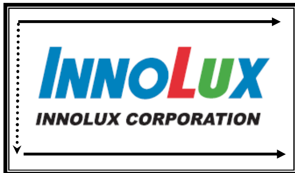
Fig. 1 Normal scan ( pin 4, LR/UD = High or NC )
